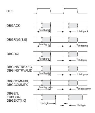
Figure 9-6 Debug interface timing
