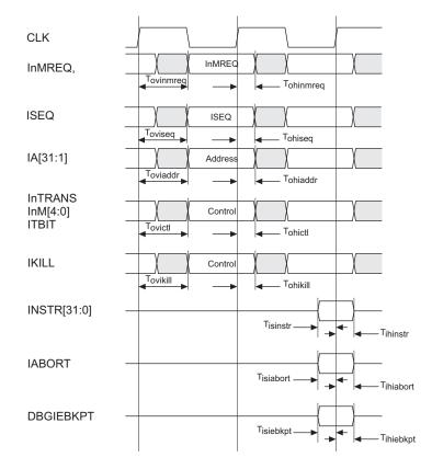
Figure 9-1 Instruction memory interface timing, InMREQ and ISEQ
