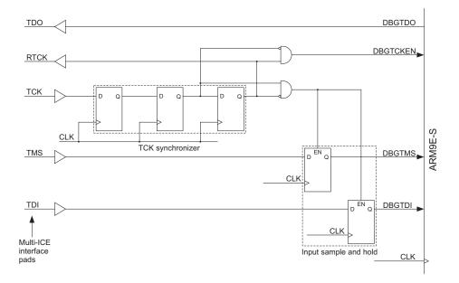
Figure 8-7 Clock synchronization
