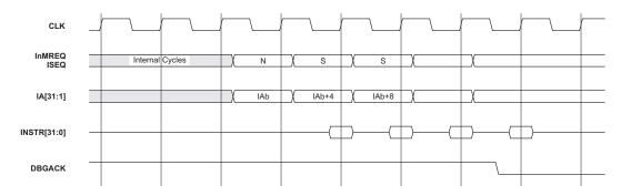
Figure B-5 shows the behavior of the ARM9E-S core on exit from debug state.
