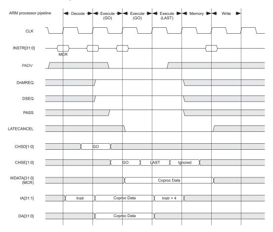
Figure 5-10 ARM9E-S core coprocessor 15 MCRs
