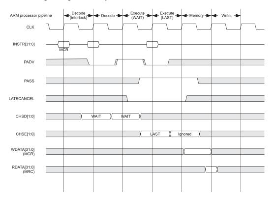
Figure 5-5 gives an example of an interlocked MCR.
