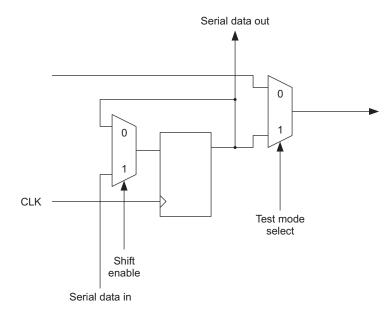
Figure B-4 Typical scan chain cell
