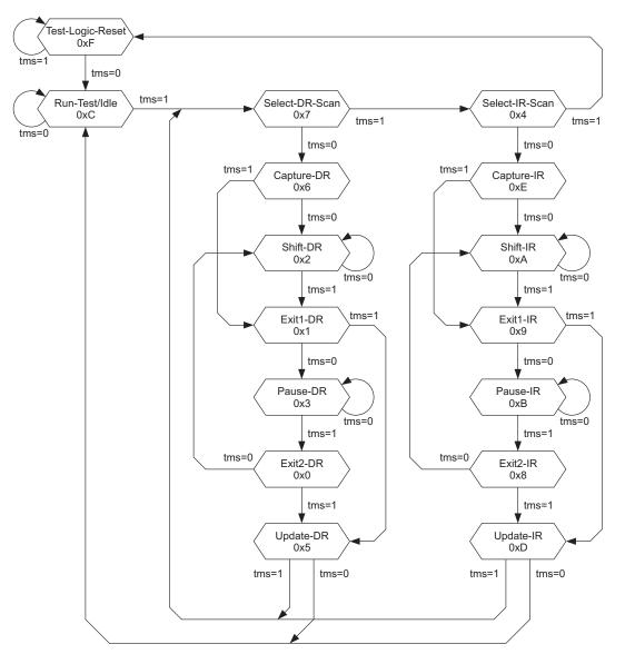
Figure B-2 Test access port controller state transitions<sup>1</sup>
