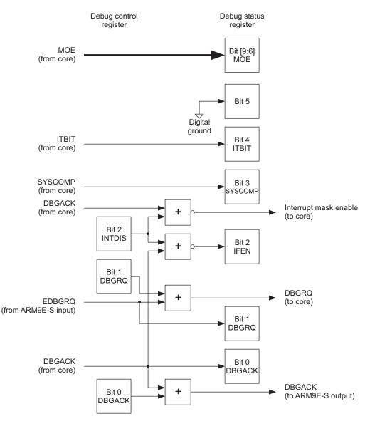
Figure B-11 Debug control and status register structure
