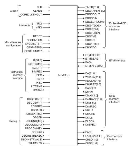
Figure 1-4 ARM9E-S interface diagram
