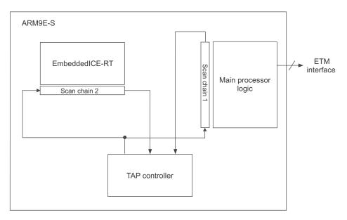
Figure B-1 ARM9E-S core scan chain arrangements
