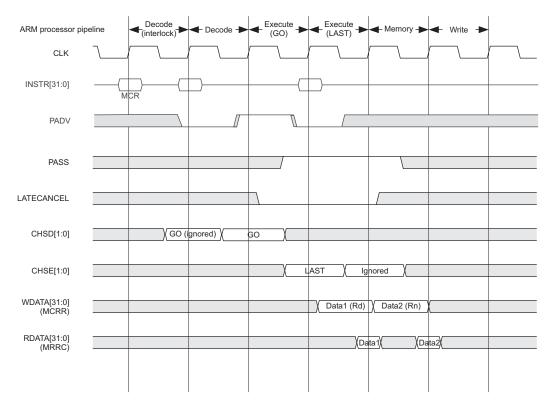
Figure 5-6 gives an example of an interlocked MCRR.
